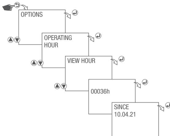
Fig. 20: Reading the operating hour counter
