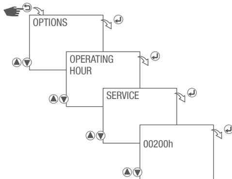
Fig. 22: Setting the service alarm
